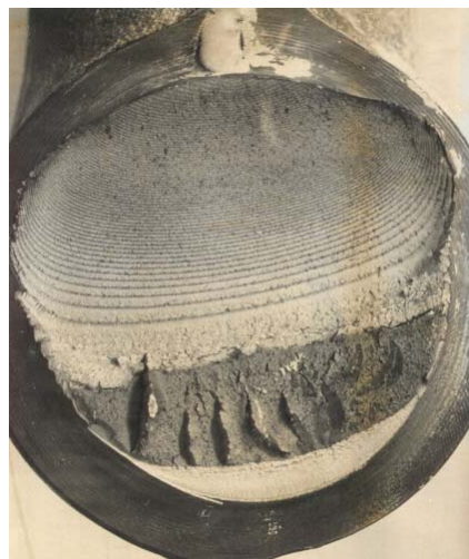
Figure 1.2 Fatigue fracture surface from a shaft in bending
