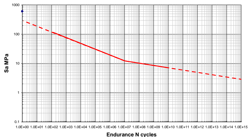
Figure 8-18 S-N curve extrapolation
