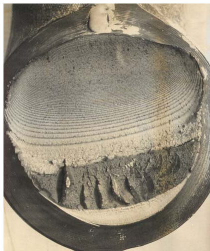
Figure 1.2 Fatigue fracture surface from a shaft in bending
